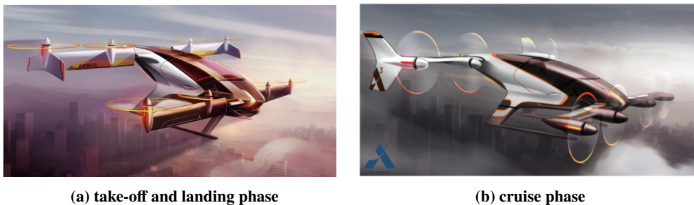
Fig. 1 Airbus Vahana with tandem tilt-wing configuration during the take-off phase and cruise phase [92].
